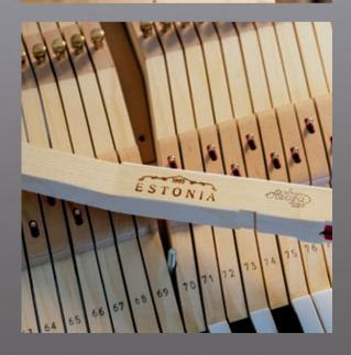
The keyboard on our piano is made to the specific instrument, as each key has been sanded, polished and weighted to achieve the optimum sensibility. Continuing the European piano-making tradition, the keybed is built into the rim, and this integrated construction of keybed, keyboard and the rim gives the piano additional stability and durability. A time-consuming process, we value the extra quality it provides to our customers.
