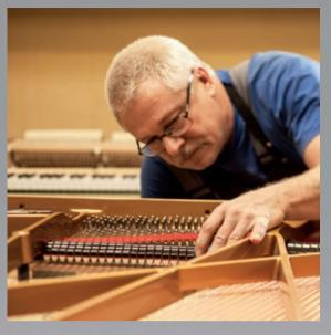
The Estonia Model 168 has a cast iron frame that has been meticulously designed to handle the high tension of the strings, ensuring stability and resonance. The cast iron frame creates the supporting structure of the instrument with outstanding workmanship, allowing the piano to reach its full potential providing captivating performances.
